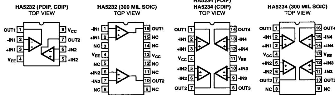
NOTE: The functional pinouts will comply to the JEDEC standards for dual and quad op amps as shown above
