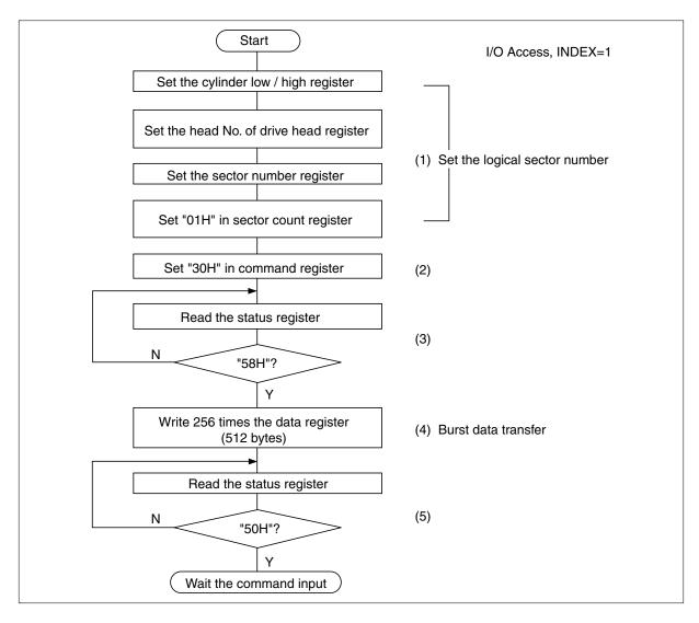
2. Sector write: 1 sector write procedure after the card configured I/O interface is shown as follows.
