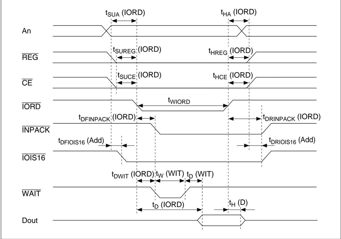
**Figure 3.7 I/O Read Timing Chart**
