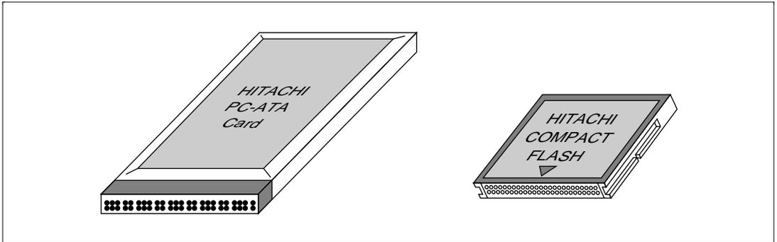
**Figure 1.1 PC-ATA Card and CompactFlash™ Outlines**
