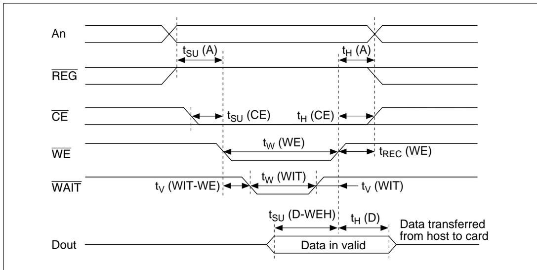
**Figure 3.6 Common Memory Write Timing Chart**
