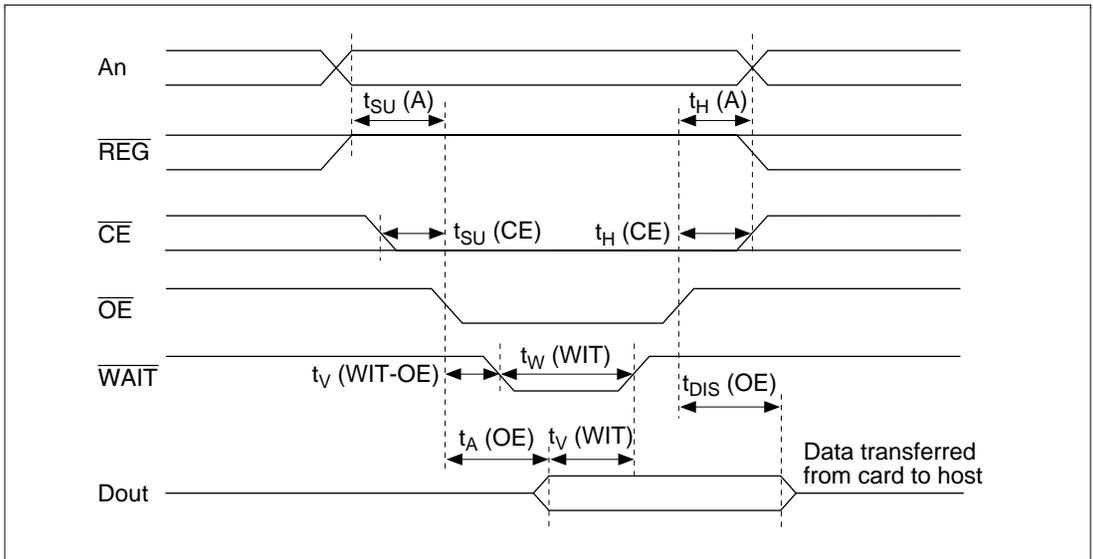
**Figure 3.5 Common Memory Read Timing Chart**
