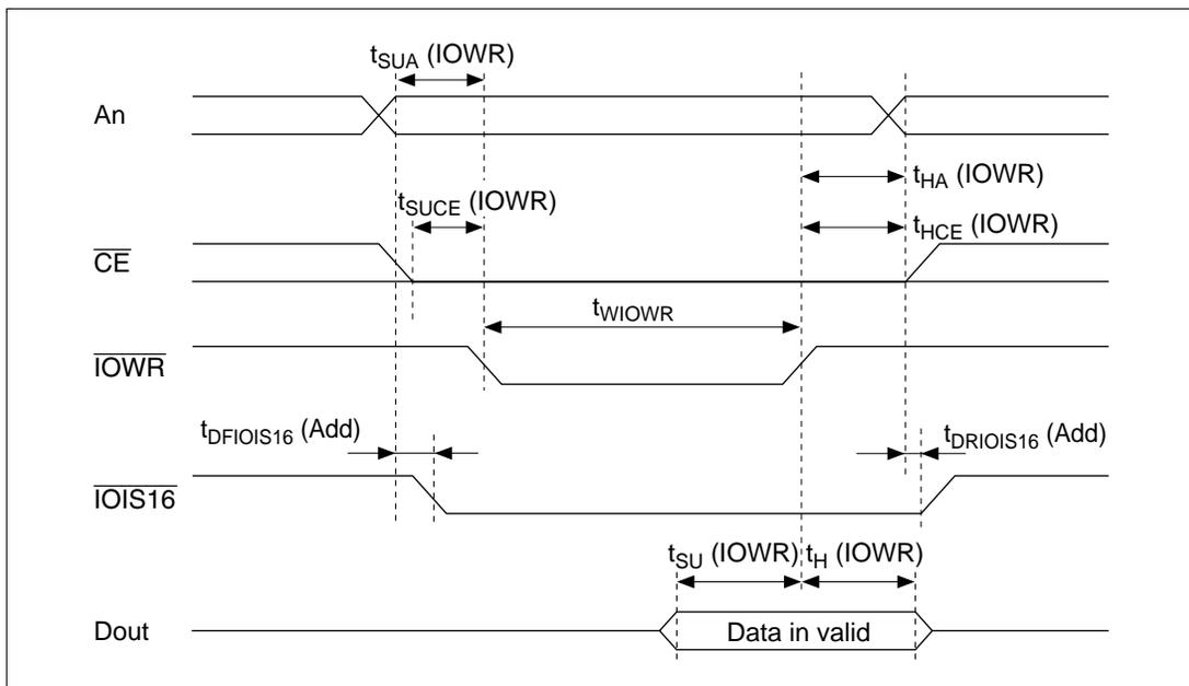
**Figure 3.10 True-IDE Write Timing Chart**
