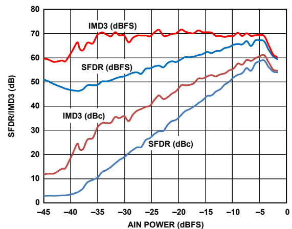
Figure 9. Two-Tone SFDR/IMD3 vs. Input Amplitude (AIN) with f_{IN1} = 29.1 MHz and f_{IN2} = 32.1 MHz
