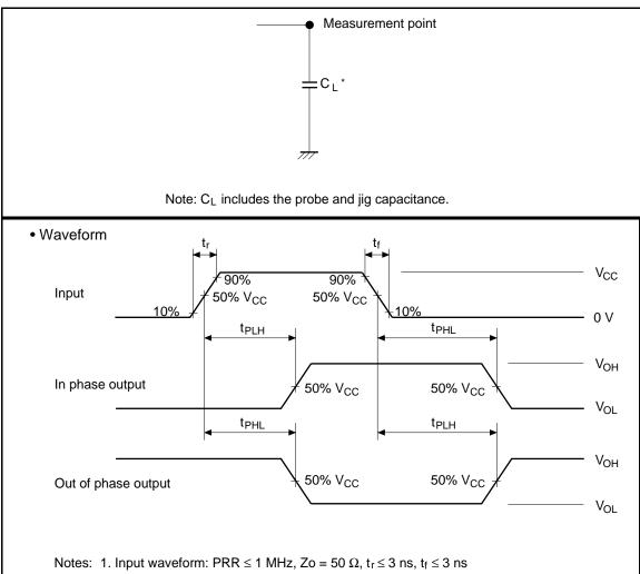
2. The output is measured one at a time with one transition per measurement.
