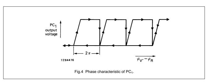
PC1 is designed to have a high gain, typically 3200 V/cycle (at 12,5 kHz). This enables a low noise performance.
