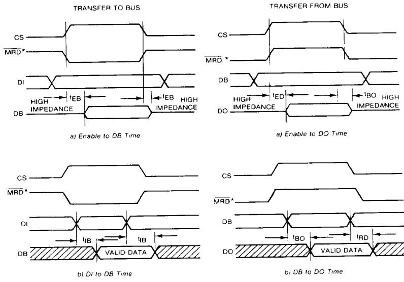
NOTE: ALL TIMES MEASURED FROM 50% POINT TO 50% POINT OF SIGNAL
