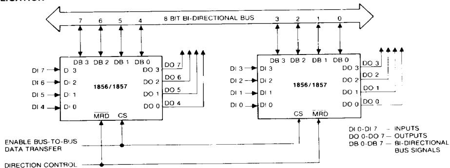
The Figure shows how two 1856 or two 1857 can be used as bus buffers or separators between an 8 Bit Bi-directional Data bus and memories or between an 8 Bit Bi-directional Data bus and I/O devices. The chip select input signal enables the bus separator three-state output drivers. The direction of data flow, when enabled, is controlled by the state of the MRD input signal.
