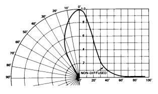
Figure 6. Relative Luminous Intensity vs. Angular Displacement.
