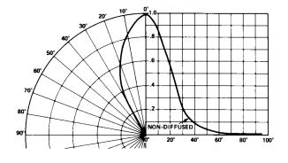
Figure 16. Relative Luminous Intensity vs. Angular Displacement.
