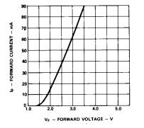
Figure 2. Forward Current vs. Forward Voltage Characteristics.
