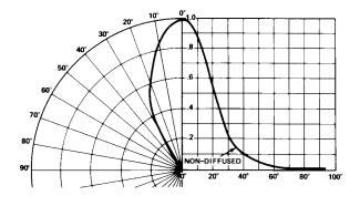
Figure 11. Relative Luminous Intensity vs. Angular Displacement.
