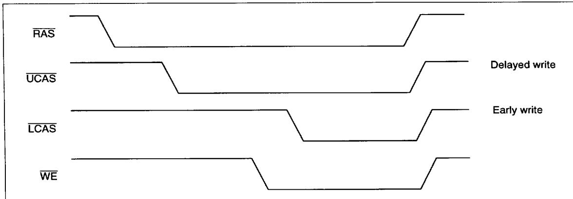
3. Closely separated upper/lower byte control is not allowed. However when the condition ( $t_{CP} \leq t_{UL}$ ) is satisfied, fast page mode can be performed.
