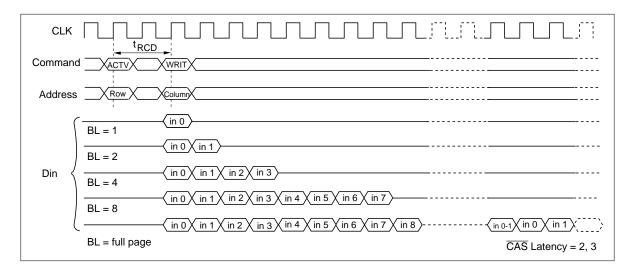
**2. Single write:** A single write operation is enabled by setting OPCODE (A9, A8) to (1, 0). In a single write operation, data is only written to the column address (AY0 to AY7; HM5264165, AY0 to AY8; HM5264805, AY0 to AY9; HM5264405) and the bank select address (A12/A13) specified by the write command set cycle without regard to the burst length setting. (The latency of data input is 0 clock).
