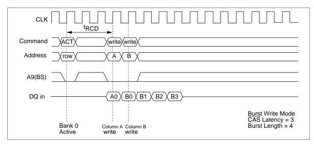
2. Operation for a column in other row of the same bank: It is necessary to execute a precharge command and a bank active command before executing the following write command.
