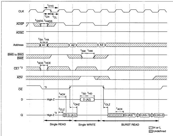
Notes: 1. Q (A3) refers to output from address A3. Q (A3 + 1) refers to output from next internal burst address following A3 2.  $\overline{\text{CE2}}$  and CE2 have timing identical to  $\overline{\text{CE1}}$ . On this diagram, when  $\overline{\text{CE1}}$  is LOW,  $\overline{\text{CE2}}$  is LOW and CE2 is HIGH. When  $\overline{\text{CE1}}$  is HIGH,  $\overline{\text{CE2}}$  is HIGH and CE2 is LOW.
