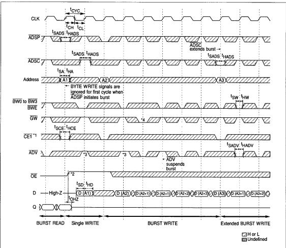
Notes: 1.  $\overline{\text{CE2}}$  and CE2 have timing identical to  $\overline{\text{CE1}}$ . On this diagram, when  $\overline{\text{CE1}}$  is LOW,  $\overline{\text{CE2}}$  is LOW and CE2 is HIGH. When  $\overline{\text{CE1}}$  is HIGH,  $\overline{\text{CE2}}$  is HIGH and CE2 is LOW.
