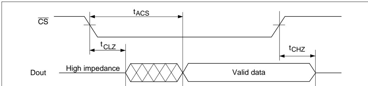
Note: 1. Address must be valid prior to or simultaneously with  $\overline{CS}$  going low.
