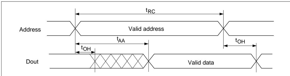
Read Timing Waveform (3) ( $\overline{WE} = V_{IH}, \overline{OE} = V_{IL}$ )\*1
