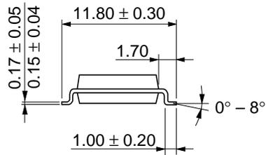
Dimension including the plating thickness
