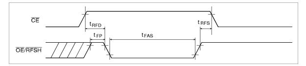
Low  $V_{CC}$  Data Retention Characteristics (Ta = -40 to +85°C)
