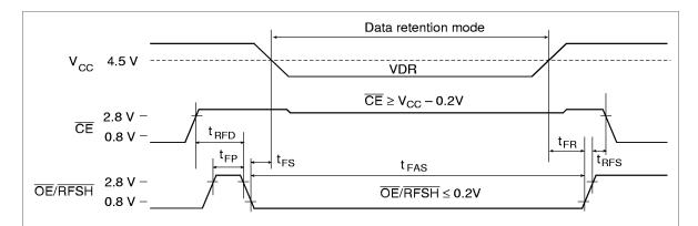
Notes: 1. Rise time and fall time of power supply voltage must be smaller than 0.05 V/ms.
