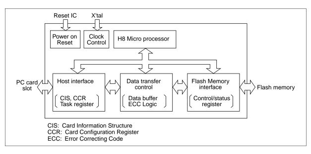
Note: The HITACHI Flash controller recover from 2-bit errors of the data field (512-byte) and 1-bit error of control field (16-byte) during read operation.
