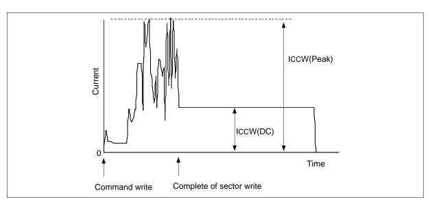
AC Characteristics (Ta = 0 to +70 °C,  $V_{cc}$  = 5 V  $\pm$  10%,  $V_{cc}$  = 3.3 V  $\pm$ 5%)
