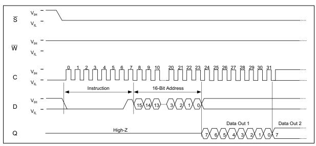
Note: 1. Depending on the memory size, as shown in the following table, the most significant address bits are don't care.
