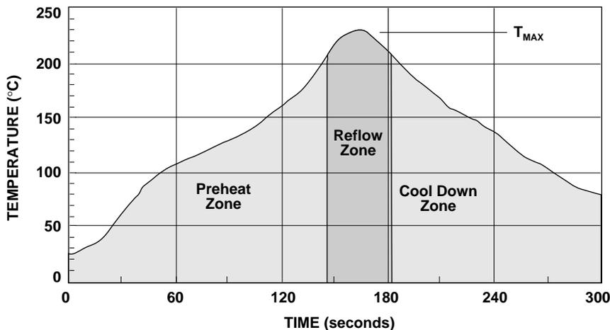
Figure 8. Surface Mount Assembly Profile.
