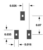
Figure 6. PCB Pad Layout (dimensions in inches).
