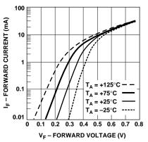
Typical Performance,  $T_C = 25^{\circ}C$  (unless otherwise noted), Single Diode
