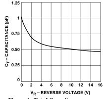
Figure 4. Total Capacitance vs. Reverse Voltage.
