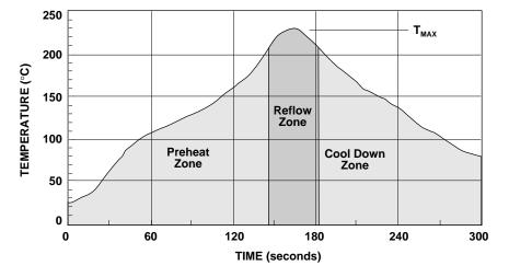
Figure 8. Surface Mount Assembly Profile.
