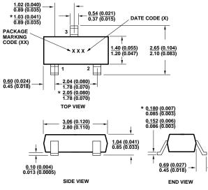
\* THESE DIMENSIONS FOR HSMS-280X AND -281X FAMILIES ONLY. DIMENSIONS ARE IN MILLIMETERS (INCHES)
