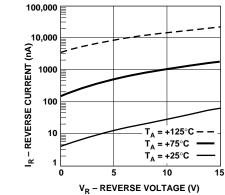
Figure 2. Reverse Current vs. Reverse Voltage at Temperatures.
