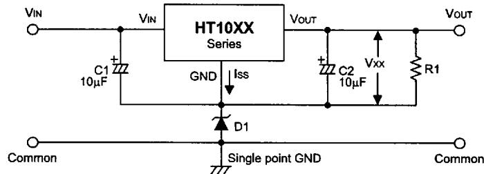
$$V_{OUT} = V_{XX} + V_{D1}$$
