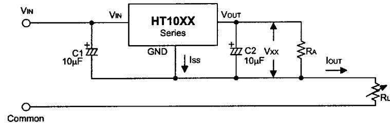
$$I_{OUT} = \frac{V_{XX}}{R_A} + I_{SS}$$
