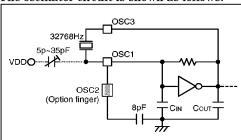
The option finger can be short-circuited by bonding to add an 8 pF capacitor to oscillator input. That is to say, if the user bonds OSC2 to pin for oscillator input, the capacitor of total input are  $C_{\rm IN}$  and 8pF (see figure). A trimmer capacitor (5pF  $\sim$  35pF) can also be connected to VDD to trim the oscillator frequency.
