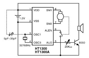
\*Note: The trimmer capacitor (5pF~35pF) is used to trim the oscillator frequency.
