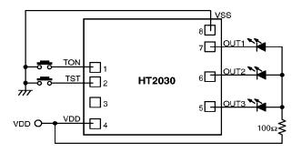
$\ensuremath{^{*}}$  The IC substrate should be connected to VDD in the PCB layout artwork.
