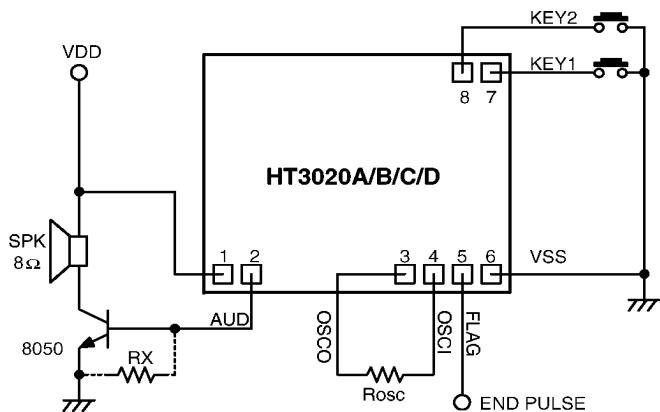
\* The IC Substrate should be connected to VSS in the PCB layout artwork.
