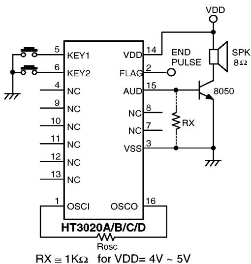
$RX \equiv 1K\Omega$  for  $VDD = 4V \sim 5V$
