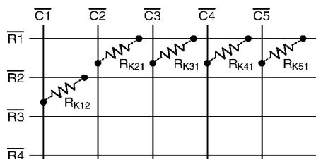
All the resistors are  $330\text{k}\Omega$ . The resistor option functions and the default specifications (without option resistors) are listed on the table.
