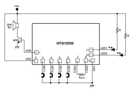
\* The IC substrate should be connected to VSS in the PCB layout artwork.
