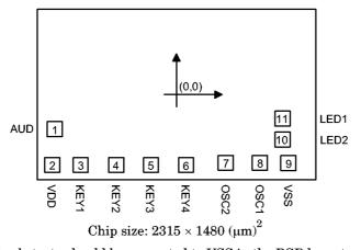
$<sup>\</sup>ensuremath{^{*}}$  The IC substrate should be connected to VSS in the PCB layout artwork.
