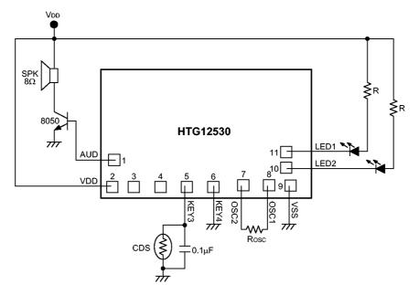
\* The IC substrate should be connected to VSS in the PCB layout artwork.
