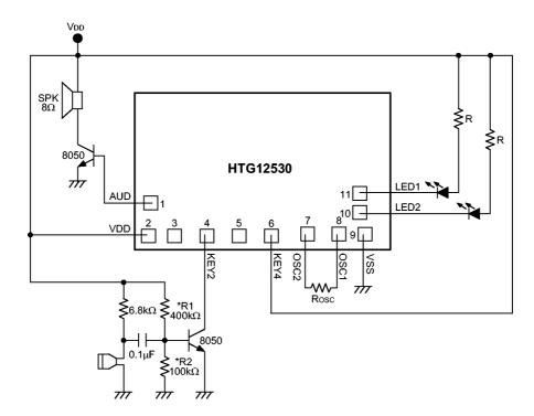
\* The IC substrate should be connected to VSS in the PCB layout artwork.
