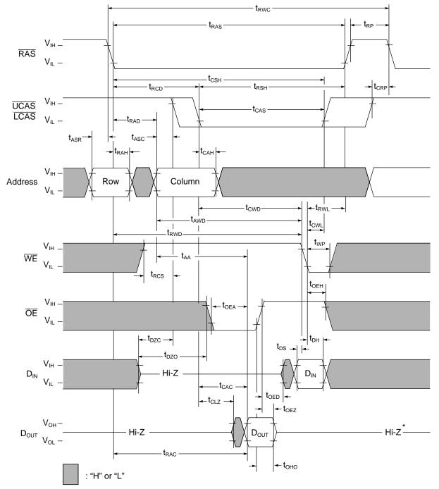
$t_{OEH}$  greater than or equal to  $t_{CWL}$
