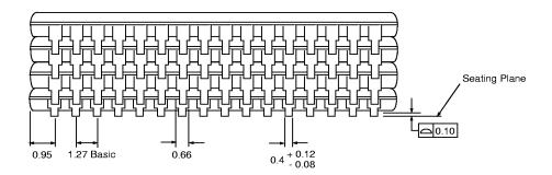
NOTE: All dimensions are in millimeters; Package Diagrams are not drawn to scale.
