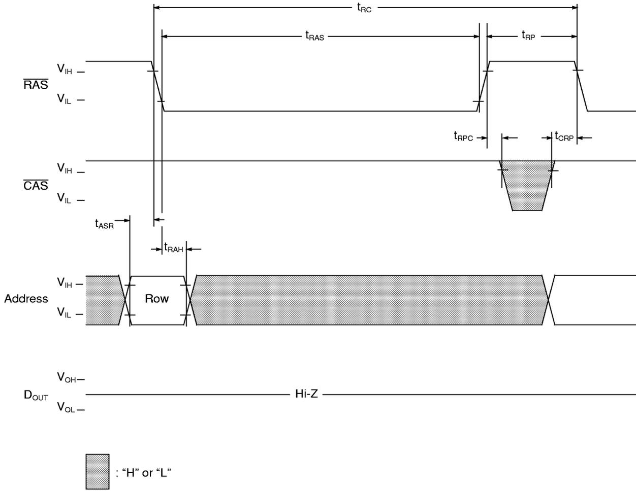
NOTE:  $\overline{\text{WE}}$ ,  $\overline{\text{OE}}$  and  $D_{\text{IN}}$  are "H" or "L"
