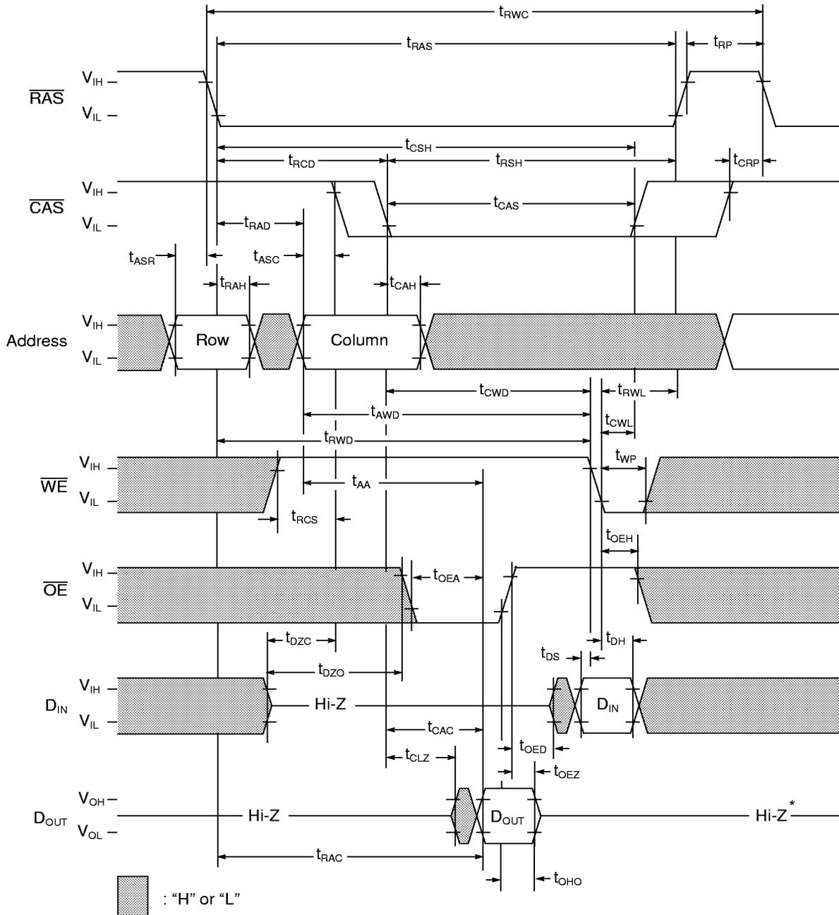
\* $t_{OEH}$  greater than or equal to  $t_{CWL}$
