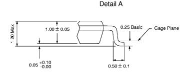
NOTE: All dimensions are in millimeters. Reference JEDEC Standard MS-24
