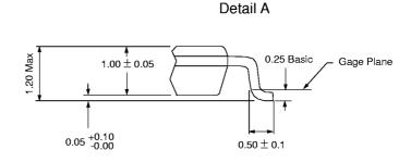
NOTE: All dimensions are in millimeters. Reference JEDEC Standard MS-024
