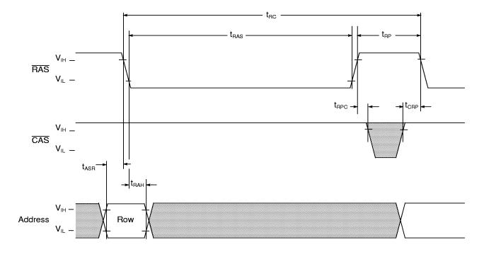
NOTE:  $\overline{\text{WE}}$ ,  $\overline{\text{OE}}$  and  $D_{\text{IN}}$  are "H" or "L"
