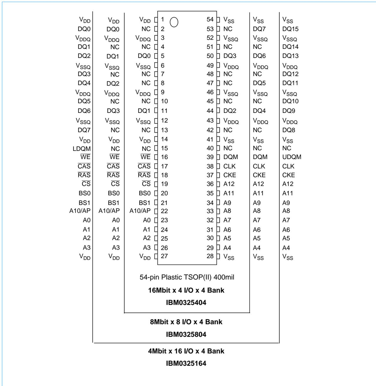
**Pin Assignments for 2 High Stack Package (Dual  $\overline{CS}$  Pin)** (Top View)
