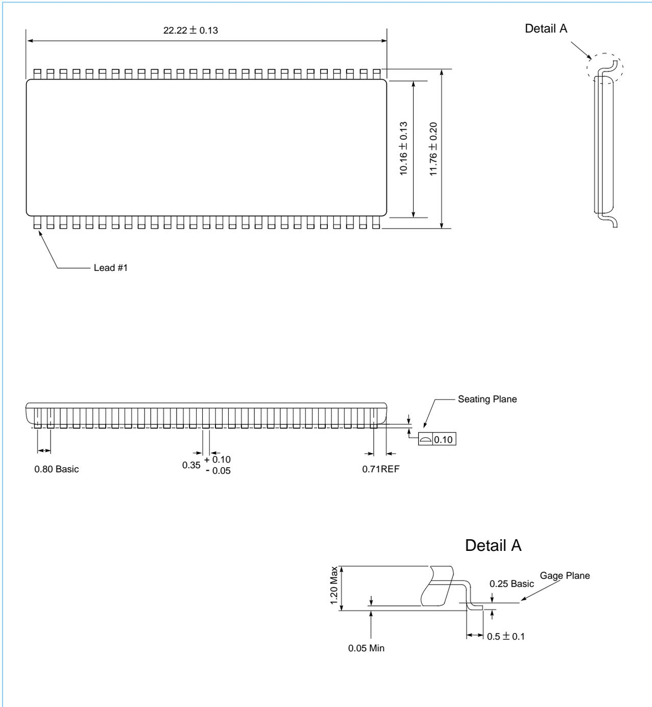
**Package Dimensions** (400mil; 66 lead; 2 High Stack; Thin Small Outline J Lead Package)
