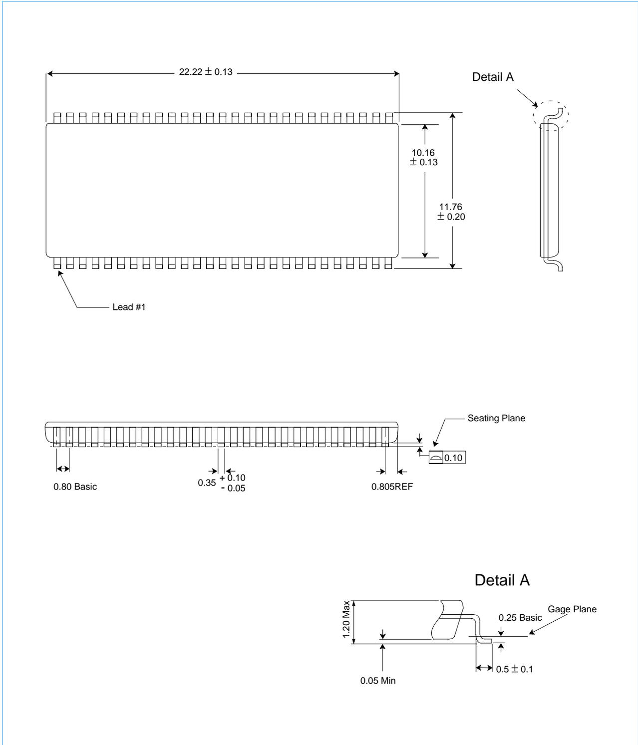
**Package Dimensions** (400mil; 54 lead; 2 High Stack; Thin Small Outline J Lead Package)
