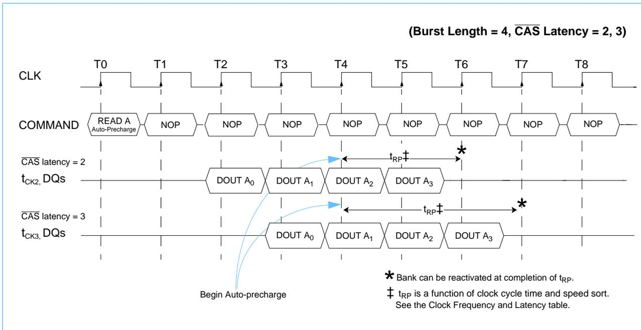
Although a Read Command with auto-precharge can not be interrupted by a command to the same bank, it can be interrupted by a Read or Write Command to a different bank. If the command is issued before auto-precharge begins then the precharge function will begin with the new command. The bank being auto-precharged may be reactivated after the delay  $t_{RP}$ .
