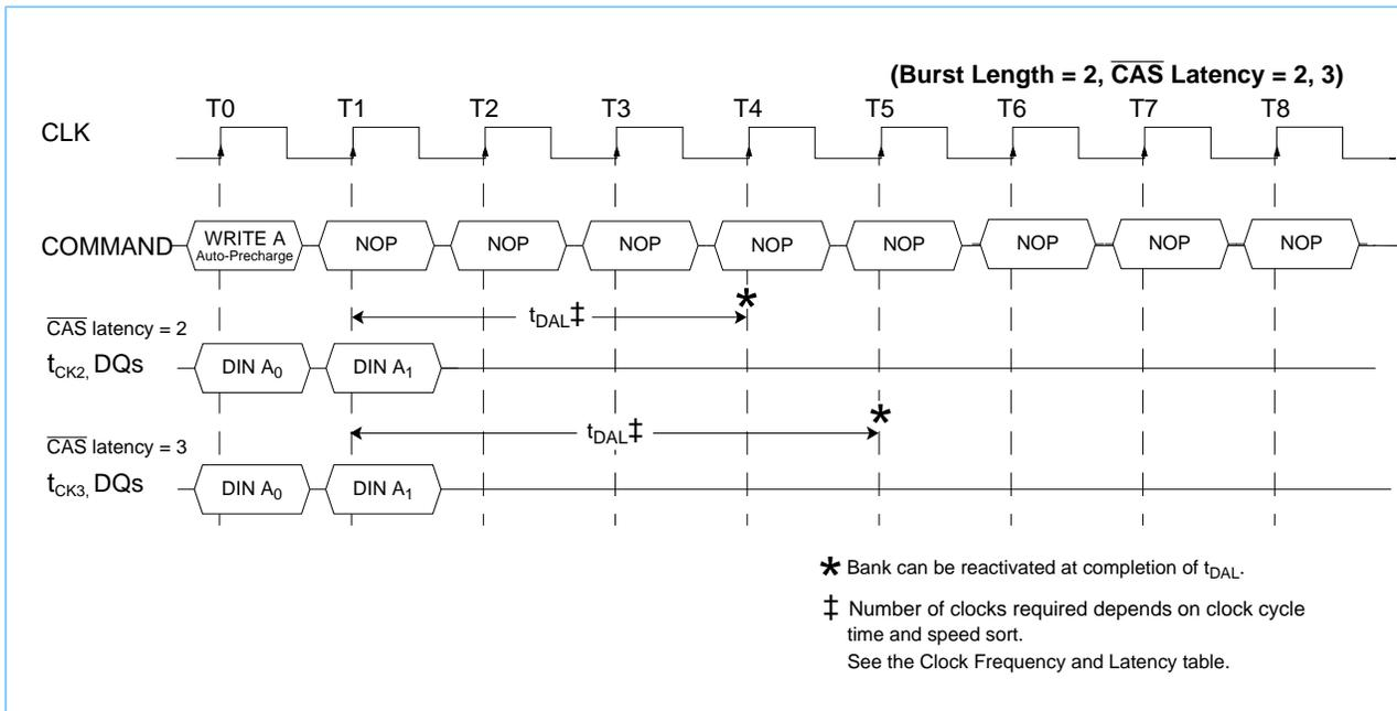
Similar to the Read Command, a Write Command with auto-precharge can not be interrupted by a command to the same bank. It can be interrupted by a Read or Write Command to a different bank, however. The pre-charge function will be initiated by the new command. After the Data-in to Active, delay,  $t_{DAL}$ , is satisfied the bank may be reactivated.
