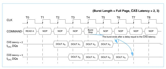
If a Burst Stop Command is issued during a full page burst write operation, then any residual data from the burst write cycle will be ignored. Data that is presented on the DQ pins before the Burst Stop Command is registered will be written to the memory.
