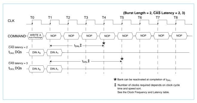
Similar to the Read Command, a Write Command with auto-precharge can not be interrupted by a command to the same bank. It can be interrupted by a Read or Write Command to a different bank, however. The precharge function will be initiated by the new command. After the Data-in to Active, delay, t<sub>DAL</sub>, is satisfied the bank may be reactivated.
