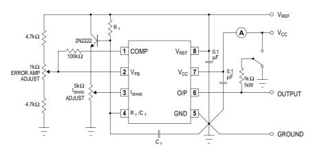
High peak current associated with capacitive loads necessitate careful grounding techniques. Timing and bypass capacitors should be connected close to pin 5 in a single point ground. The transistor and 5K potentiometer are used to sample the oscillator wave form and apply an adjustable ramp to pin 3.
