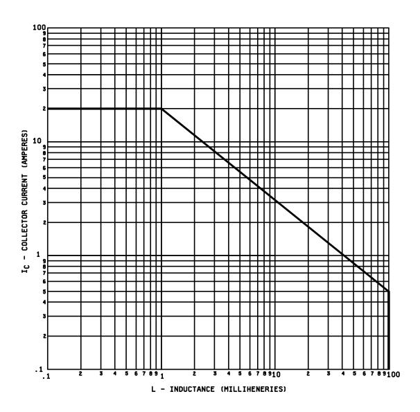
FIGURE 4. <u>Safe operating area for switching between saturation and cutoff (unclamped inductive load)</u>.
