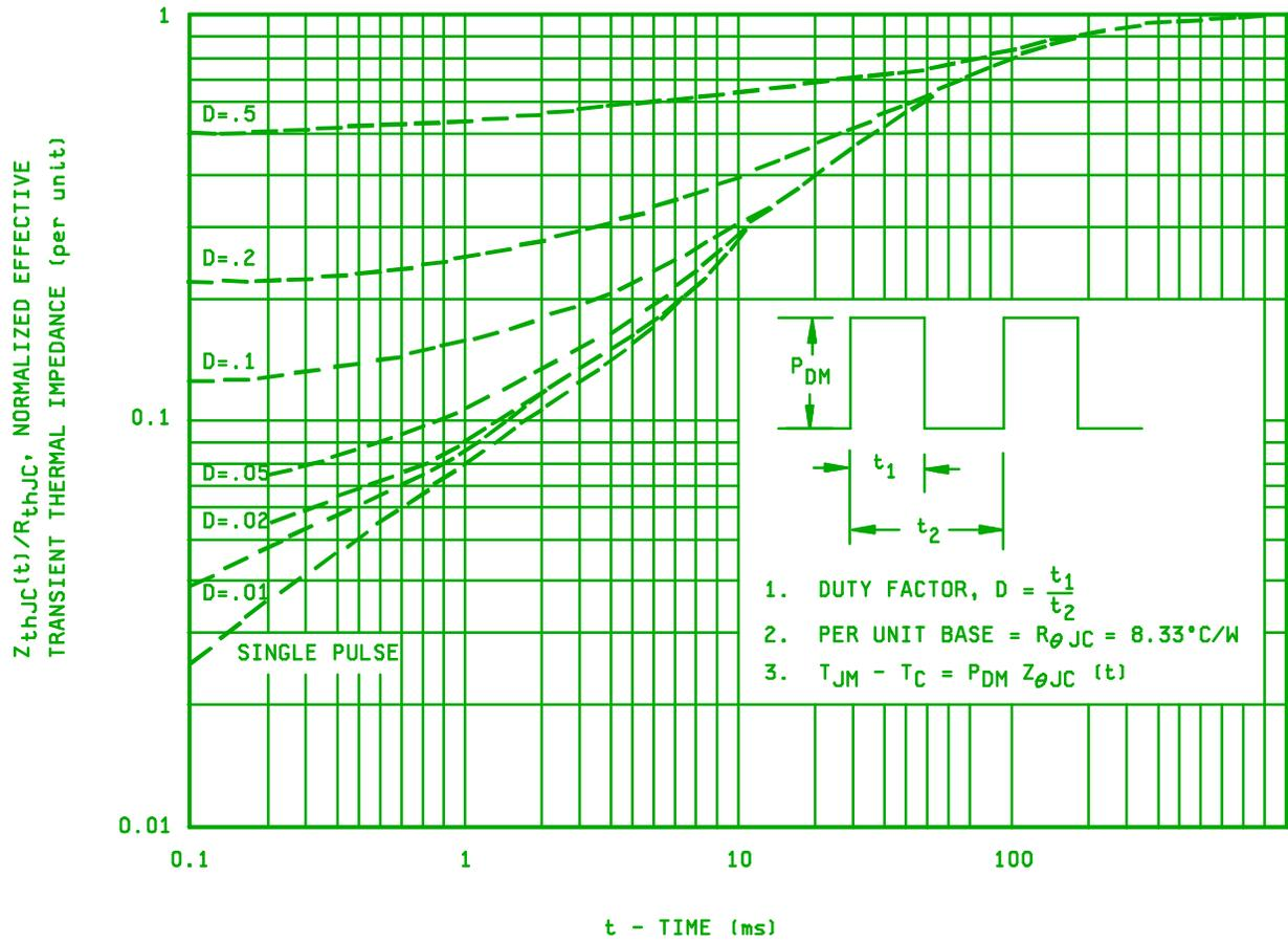
FIGURE 7. Normalized transient thermal impedance.
