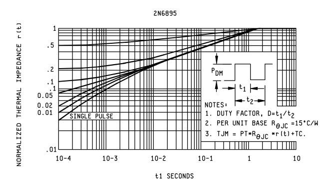
FIGURE 3. Transient thermal response.
