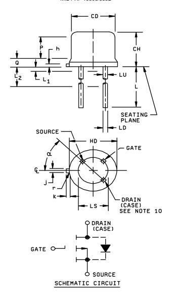
FIGURE 1. Physical dimensions for 2N6895 (TO-205AF).
