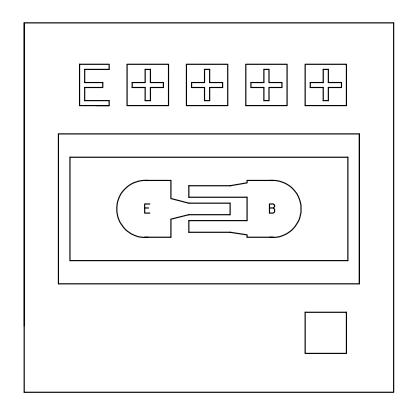
Die size:  $.016 \times .016$  inch  $(0.4064 \times 0.4064 \text{ mm})$ . Die thickness:  $.008 \pm .0016$  inch  $(0.2032 \pm 0.04064 \text{ mm})$ . Base pad:  $.0027 \times .0027$  inch  $0.06858 \times 0.06858$  mm).
