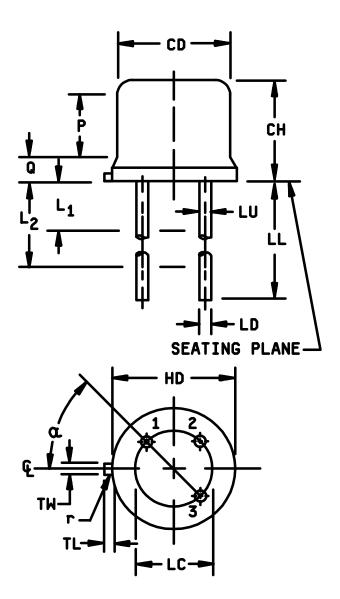
FIGURE 1. Physical dimensions for (TO-39).
