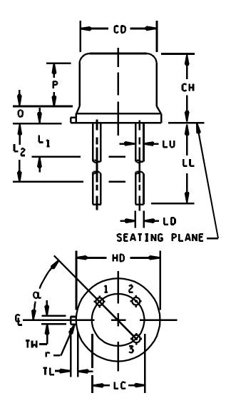
FIGURE 1. Physical dimensions for (TO-39).
