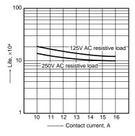
5-(2). Electrical life test Sample: JL1aZF-TMP1-12V, 5 pcs. Load: AC 125 V, 12 A Opetation frequency: 20 cpm (ON:OFF = 1.5s:1.5 s) Ambient temperature : 80°C 176°F
