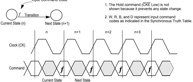
Current State and Next State Definition for Pipelined and Flow through Read/Write Control State Diagram
