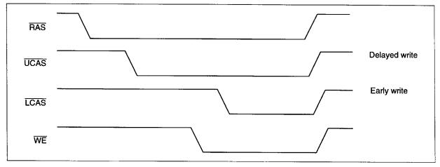
3. Closely separated upper/lower byte control is not allowed. However when the condition  $(t_{CP} \le t_{UL})$  is satisfied, EDO page mode can be performed.
