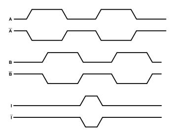
Waveforms for Encoders with Line Drivers. (Meets all requirements of EIA-422.)
