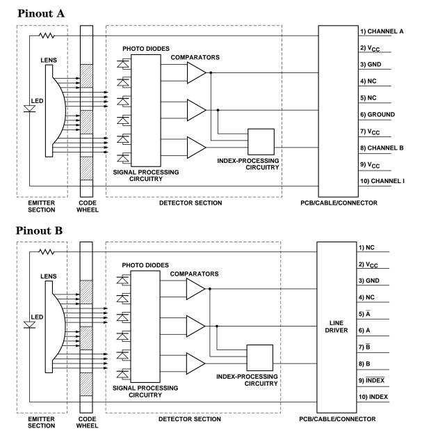
There are two different connector pin-out configurations used with the HEDS-65xx / HEDL-65xx series of encoders. The table below relates the part to its connector pin-out.
