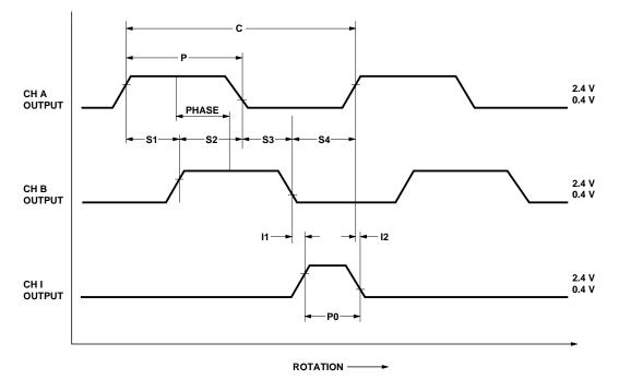
Waveforms for Encoders without Line Drivers.
