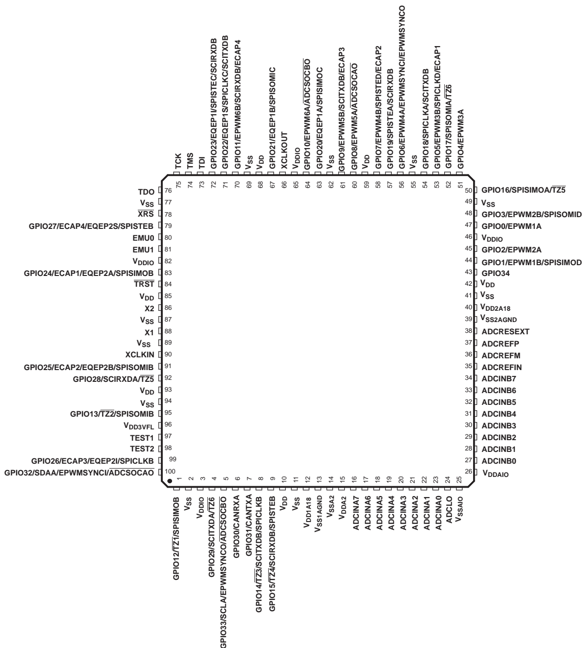
Figure 2-2. TMS320F2806 100-Pin PZ LQFP (Top View)
