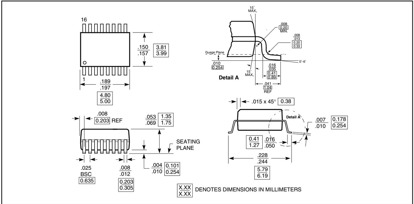
Packaging Mechanical: 16-pin SOIC (W)
