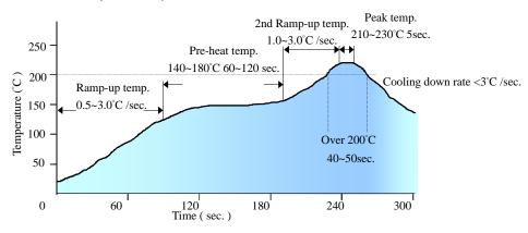
Note: The temperature refers to the pin of E48SH, measured on the pin +Vout joint.
