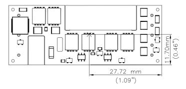
**Figure 21:** Case temperature measurement location. Pin locations are for reference only. \*The allowed maximum hot spot temperature is defined at 130  $^{\circ}$ C
