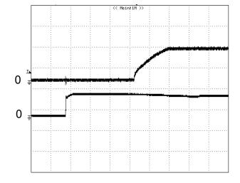
**Figure 6:** Turn-on transient at zero load current (2 ms/div). Vin=48V.Top Trace: Vout, 1V/div, Bottom Trace: input voltage, 5V/div
