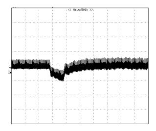
**Figure 8:** Output voltage response to step-change in load current (75%-50% of Io, max; di/dt = 0.1A/µs). Load cap: 10µF, tantalum capacitor and 1µF ceramic capacitor. Trace: Vout (20mV/div, 100us/div), Scope measurement should be made using a BNC cable (length shorter than 20 inches). Position the load between 51 mm to 76 mm (2 inches to 3 inches) from the module..
