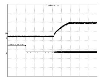
**Figure 4:** Turn-on transient at zero load current (5 ms/div). Vin=48V.Top Trace: Vout, 1V/div; Bottom Trace: ON/OFF input, 5V/div
