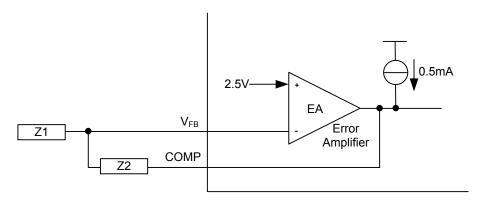
Note: Error amplifier can source or sink up to 0.5mA.
