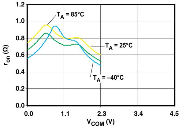
Figure 1.  $r_{on}$  vs  $V_{COM}$  ( $V_+ = 2.25$  V)
