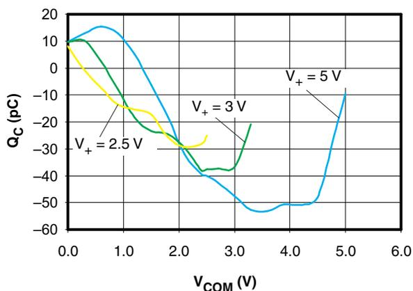
Figure 9. Charge Injection ( $Q_C$ ) vs  $V_{COM}$
