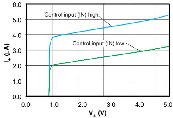
Figure 5.  $I_+$  vs  $V_+$  ( $T_A = 25^\circ\text{C}$ )
