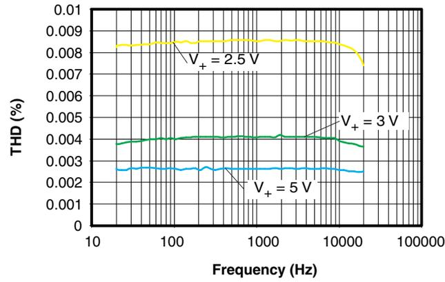
**Figure 13. Total Harmonic Distortion (THD) vs Frequency**
