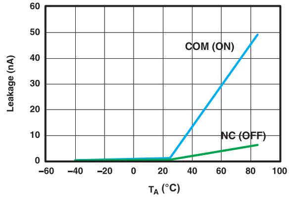
Figure 4. Leakage Current vs Temperature ( $V_+ = 5$  V)
