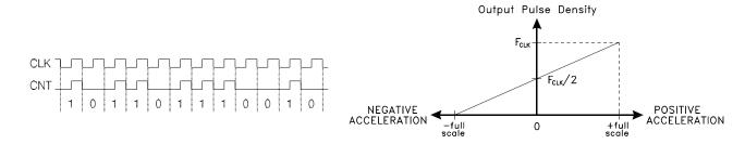
Pulses from the **CNT** output are meant to be accumulated in a hardware counter. Each pulse accumulation or sample, reflects the average acceleration (change in velocity) over that interval. The sample period or "gate time" over which these pulses are accumulated determines both the bandwidth and quantization of the measurement.
